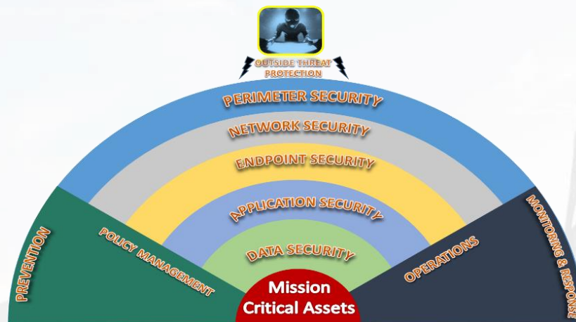
Figure 13.11: Cyber-Security Protection Layers
