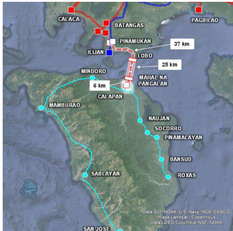
Figure 13.3: Batangas–Mindoro Interconnection Project
