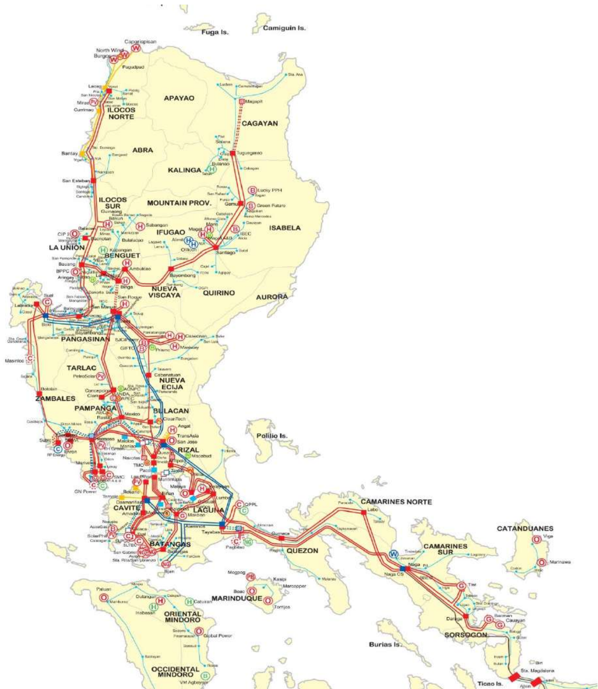
Figure 3.3: Luzon Transmission Network
